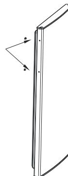
Step 2: Install the door handle to the door and fasten it with screws
