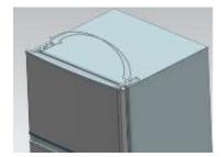
10) Set the top door right position, fix the top-hinge and the cover.
