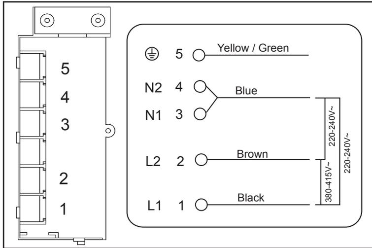
If the total number of heating unit of the appliance you choose is not less than 4, the appliance can be connected directly to the mains by single-phase electric connection, as shown below.
