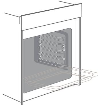
Bakeing tray- glass is installed in the same position as Baking Tray(optional accessories)
