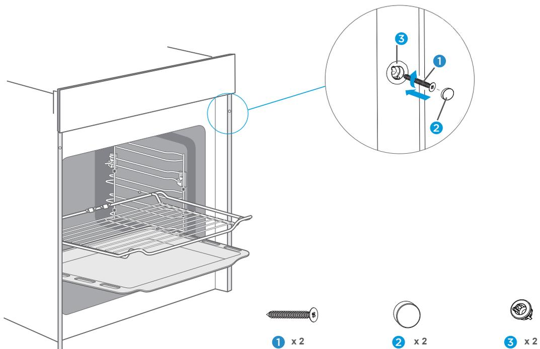
Once the oven has been lifted into place inside the appliance housing, locate the two holes in the casing of the oven and fix it into place using 1 , 2 and 3 .
